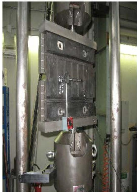
Vertical deflection measured at the centre of the profile of the test specimen of joints is reported in the Table below.
